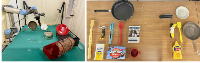
Figure 5: Our setup. We have a Realsense D455 camera, During our tests, we use a large number of background objects such as the two dish racks and the wooden chest to reflect a real world scenario. The right image shows all objects used in experiments. Left side are novel objects, right side are original objects.
